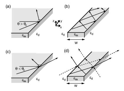
FIG. 1. Simple ray optics schematics for the modes of a metal stripe waveguide. Total internal reflection of a surface polariton wave, (a), may lead under proper interference conditions to a guided surface polariton mode, (b). Surface polariton waves may also be transmitted, (c), which necessarily leads to a radiation mode (d). Note that the radiation mode must appear to have a source outside of the waveguide to be an eigenmode of the system, as depicted by the dashed lines.
