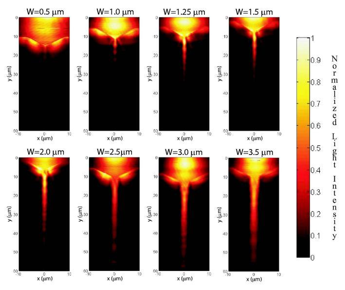
FIG. 3. (Color online) Experimental near-field images of surface plasmon propagation along varying width metal stripe waveguides ranging from 0.5  $\mu$ m to 3.5  $\mu$ m.
