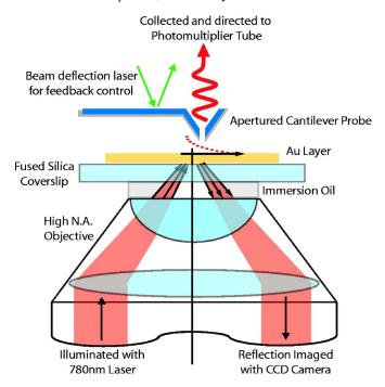
FIG. 2. (Color online) Schematic of photon scanning tunneling microscope (PSTM). A partially illuminated high numerical aperture objective is used to excite surface plasmon-polaritons along the Au-Air interface via attenuated total reflection. Light is scattered from these surface waves by an aperture cantilever probe and detected by a photomultiplier tube. Note that the sample and illumination objective are rigidly mounted to a x, y, z piezostage which is scanned below the fixed cantilever.
